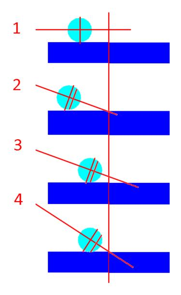
It follows that a ball on disc test machine designed with the ball rotational axis horizontal (1) will create a contact that combines both rolling, with or without slip in the rolling plane, and spin. At zero slide-roll ratio, this contact will generate traction, because of the spin component.
