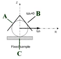
If the ball is running in a straight line on the fixed sample, in other words, rotating about the axis R, then contact C will have pure rolling but contacts A and B will be subjected to "spin" in the contact. In this case, failure will occur at either contact A or B before C, hence as a test assembly, this will only work as a device for testing rolling contact fatigue in a contact with spin, not pure rolling!
