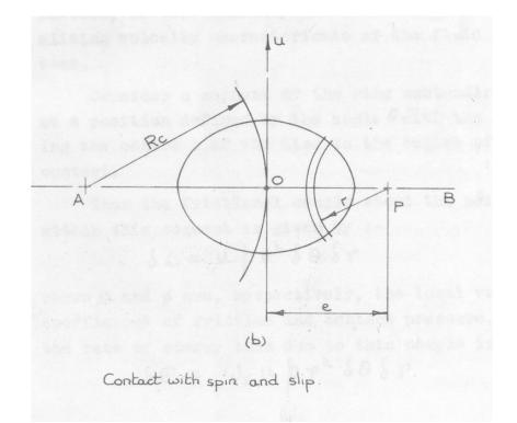
It is not what the ball is doing, it is what is happening in the hertzian contact that counts and the only way to analyse spin is to look at the velocity vectors within the contact. If they are all straight and parallel, there is no spin. If they are not, then there is either spin or skew, or frequently, both.
